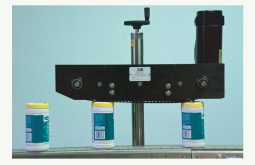
The Certified Machinery Cap Press unit is designed to bolt onto a customer's existing conveyor line and allows a cap to be pressed/applied into position on a mating component while in motion. It can also be used as a stabilizing device on tall or unstable products prior to other packaging operations.
