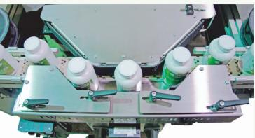
Conveyor mounted Twin Belt Diverter Unit for accessing underside of containers for bottom ink jet coding applications. The unit is designed to be used when it is not convenient to create a break in the line and can be easily mounted to most conveyors. Adjustments for varying container sizes takes only minutes. Variable speed synchronized drive ensures correct speed matching.
